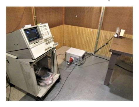
Radiated Emissions Test Setup Pictures
