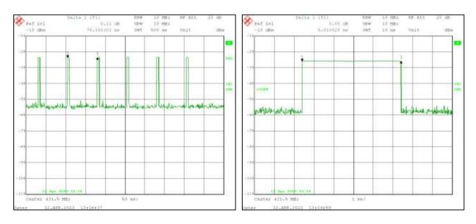
The measured on-times depicted on the spectrum analyzer screens above are used to calculate the Duty Cycle Correction Factor. This factor is used to reduce the emission level of spurious emissions measured and displayed in Section 4.3.
