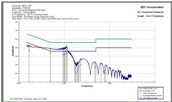
**Results:** The Lutron Models DS-5ANS / DVRF-5NS Samples 2197-01 and 2197-02 comply with the requirements of FCC Part 15.207 and RSS-Gen Section 8.8. The margin is 1.14 dB @ 504.772 kHz with Sample #2197-01 transmitting Low Channel, 431.5 MHz, Neutral Line.
