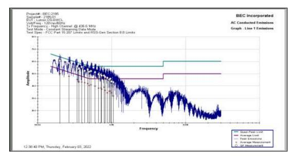
**Results:** The Lutron Model DS-6WCL Vogelkop RF Wireless Dimmer, BEC Sample #2185-02 complies with the requirements of FCC Part 15.207 and RSS-Gen Section 8.8. The margin is 3.25 dB @ 473.64 kHz on Line 1.
