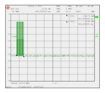
TX FREQUENCY OF 436.6 MHZ FCC PART 15.231(a)(1) RSS-210 A.1.1(a) 5 SECOND DEACTIVATION
