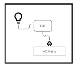
Note: conducted setup is the same with the exceptions being the lightbulb is not present and antenna port is connected directly to spectrum analyzer.
