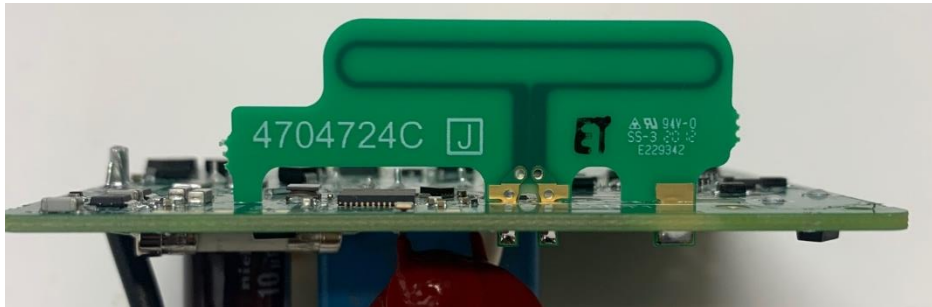
SIDE VIEW OF ANTENNA BOARD
