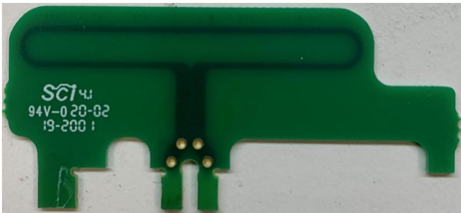
Back of Antenna Board
