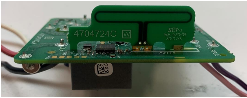
Side View of Antenna Board
