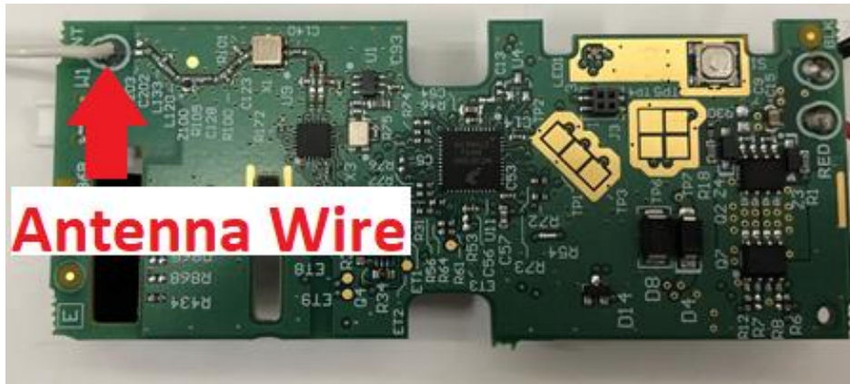
Interior (RF Antenna)
