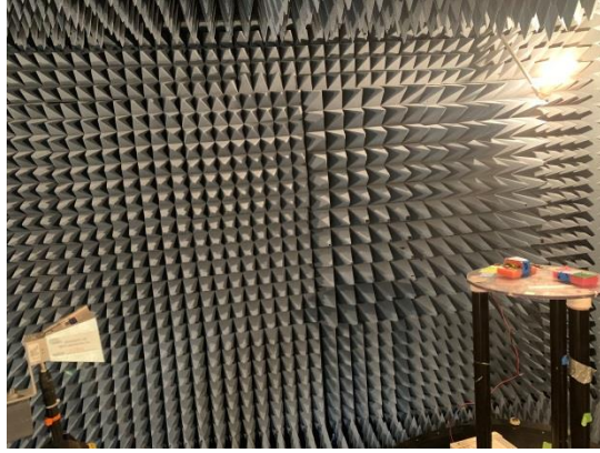
Figure 7: Radiated Emissions, Test Setup, 18 -25 GHz Antenna 2
