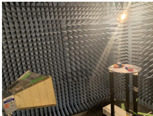
Figure 5: Radiated Emissions, Test Setup, Above 1 GHz Antenna 2
