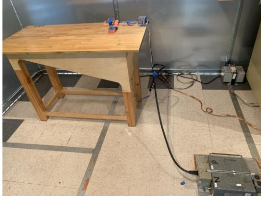
Figure 1: Conducted Emissions, Test Setup
