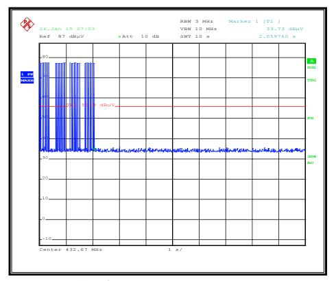
The device stops transmitting after 2.06s.
