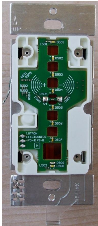
GT-RF Antenna Removed
