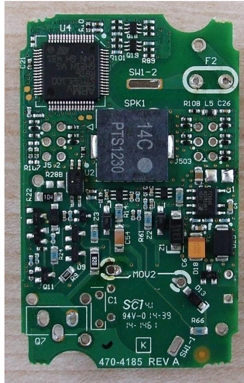
GT-RF-Front of Power Board
