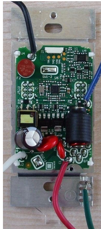
GT-RF Back of power board
