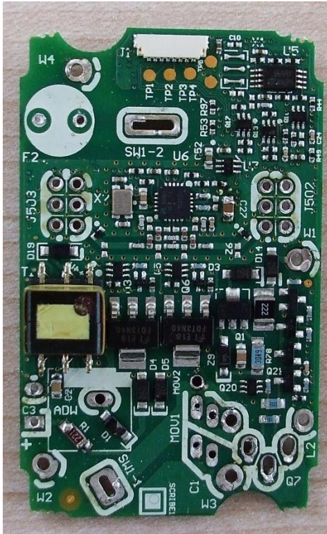
GT-RF Back of Power board
