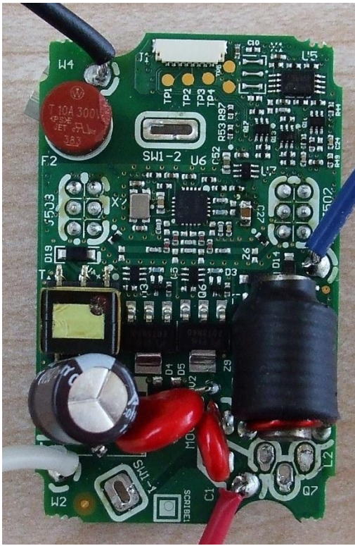
GT-RF Back of Power Board
