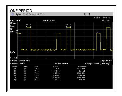
NOTE: Lower level pulses are from triggering device for repeater to start transmission.
