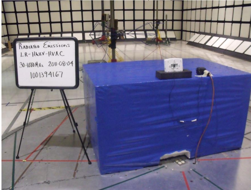
RADIATED EMISSIONS ABOVE 30 MHz (BACK)
