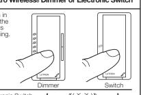
Add the Sensor to the Dimmer or Electronic Switch by pressing and holding the "Lights Off" button on the front of the Sensor for approximately 6 seconds until the lens flashes briefly. The lights in the room will also flash 3 times, indicating the Sensor has been successfully added. The Dimmer or Electronic Switch will exit set-up mode automatically.
