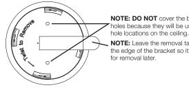
NOTE: Leave the removal tab exposed past the edge of the bracket so it can be accessed for removal later.
