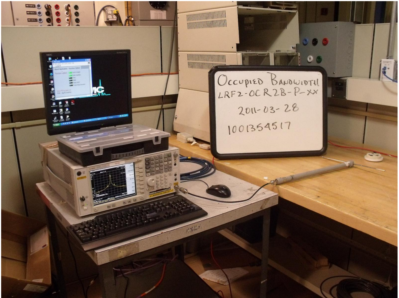
Figure 1 Test Setup for Occupied Bandwidth
