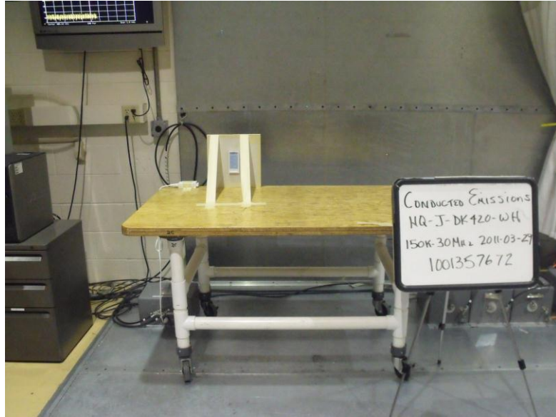
Figure 1 Test Setup for Conducted Emissions
