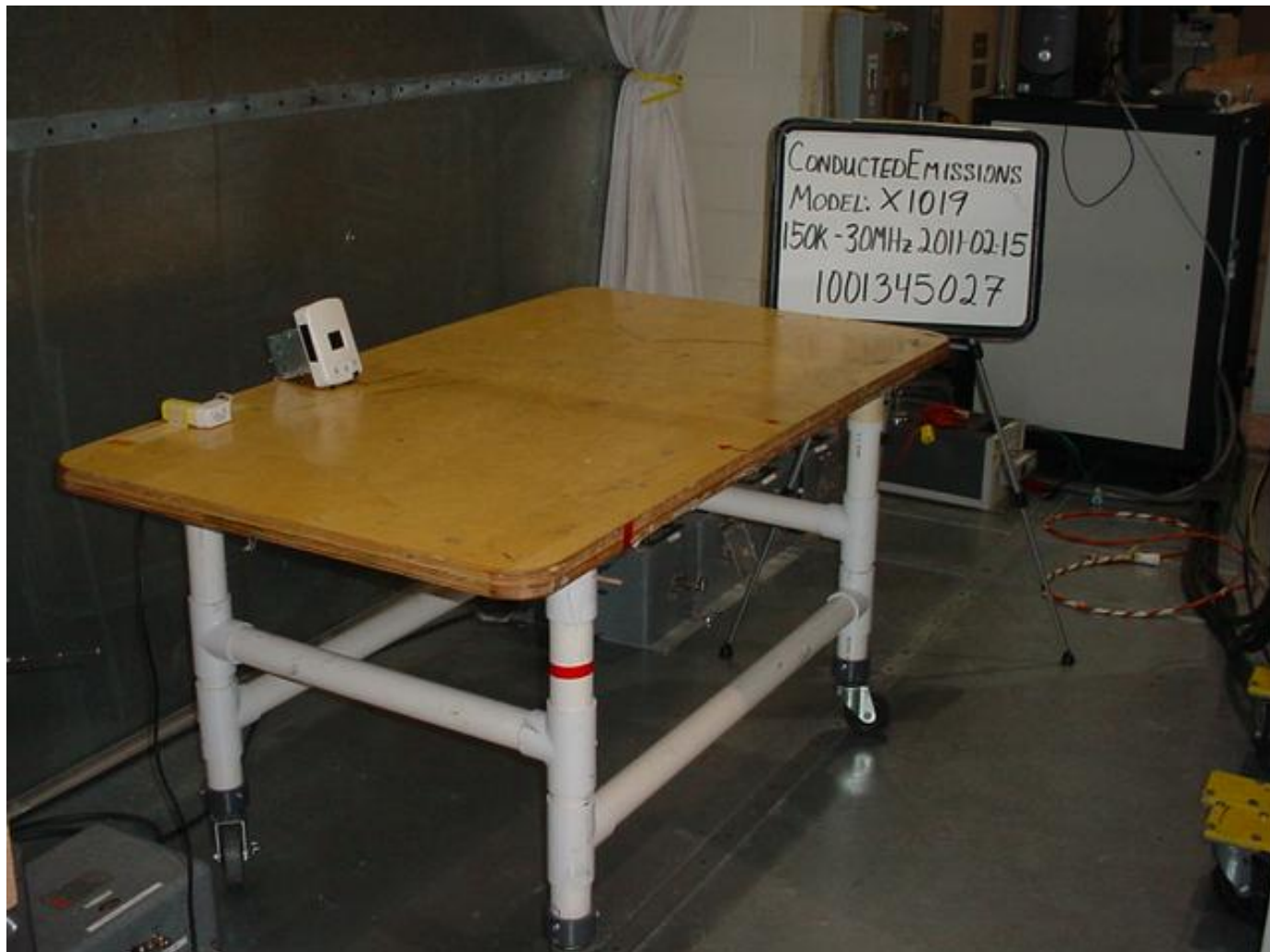
Figure 1 Test Setup for Conducted Emissions
