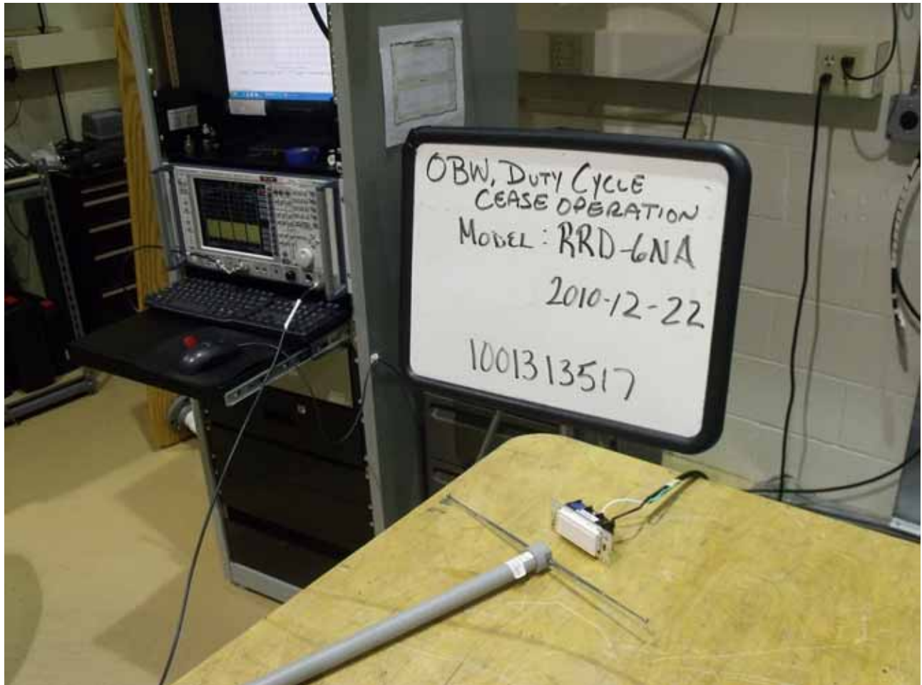
Figure 6 Test Setup for Occupied Bandwidth
