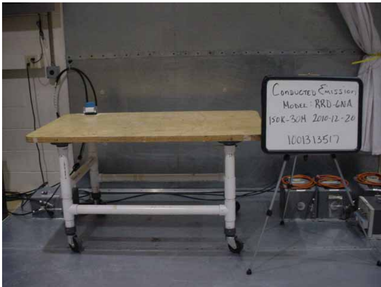
Figure 1 Test Setup for Conducted Emissions
