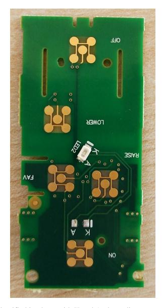
Note: LED2 may be placed in either location, identified in photo with K and A, depending on button configuration.
