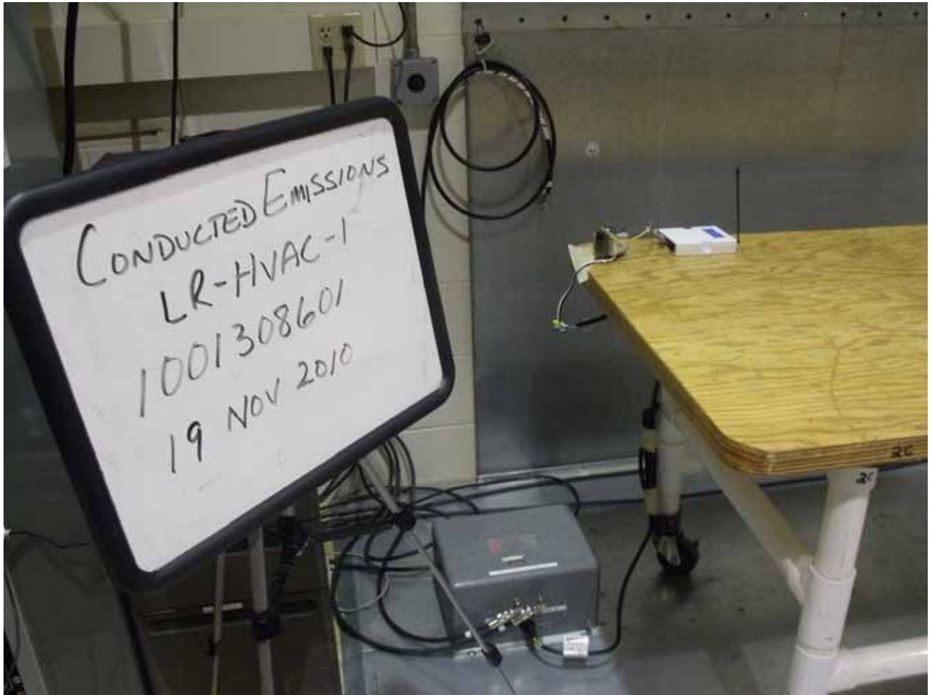
Figure 1 Test Setup for Conducted Emissions
