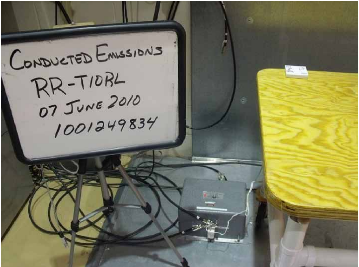
Figure 1 Test Setup for Conducted Emissions
