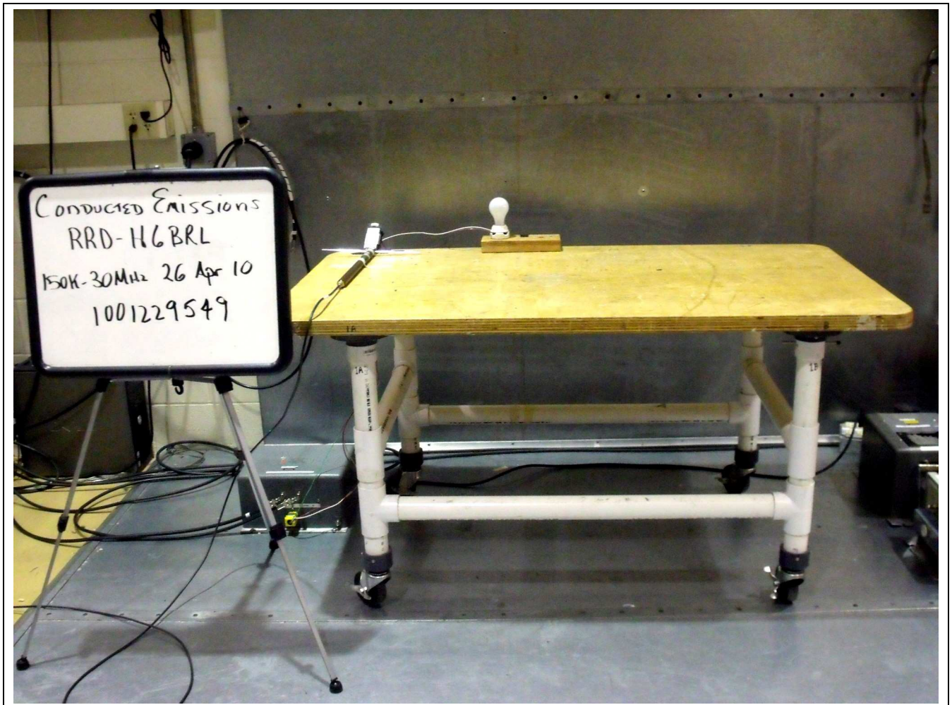
Figure 1 Test Setup for Conducted Emissions
