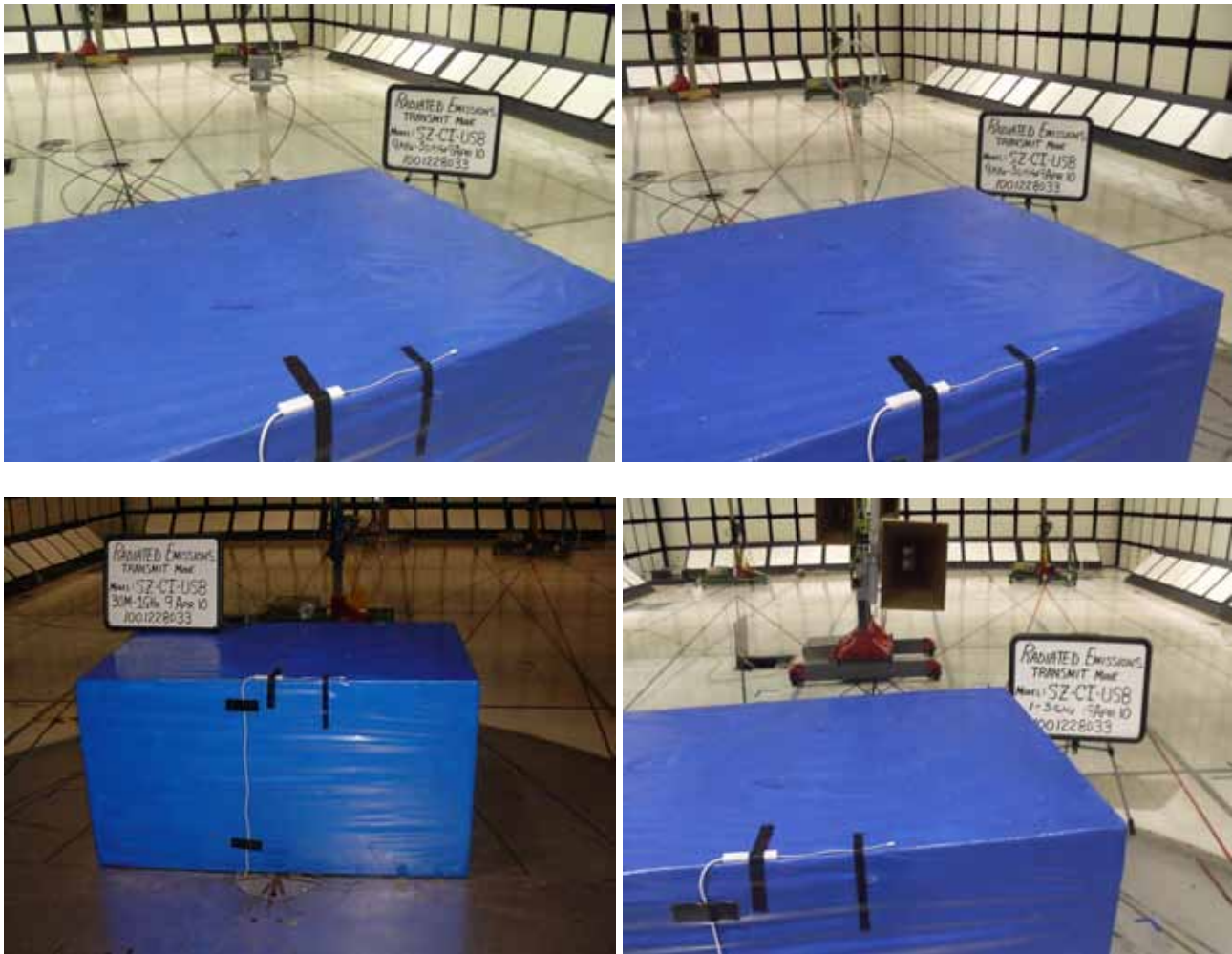
Figure 13 Test setup for Radiated Emissions
