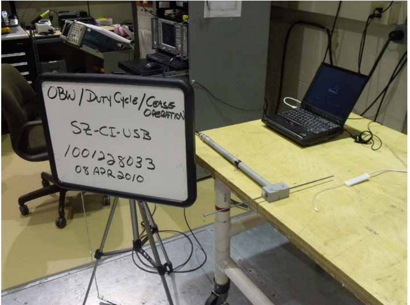
Figure 6 Test Setup for Occupied Bandwidth
