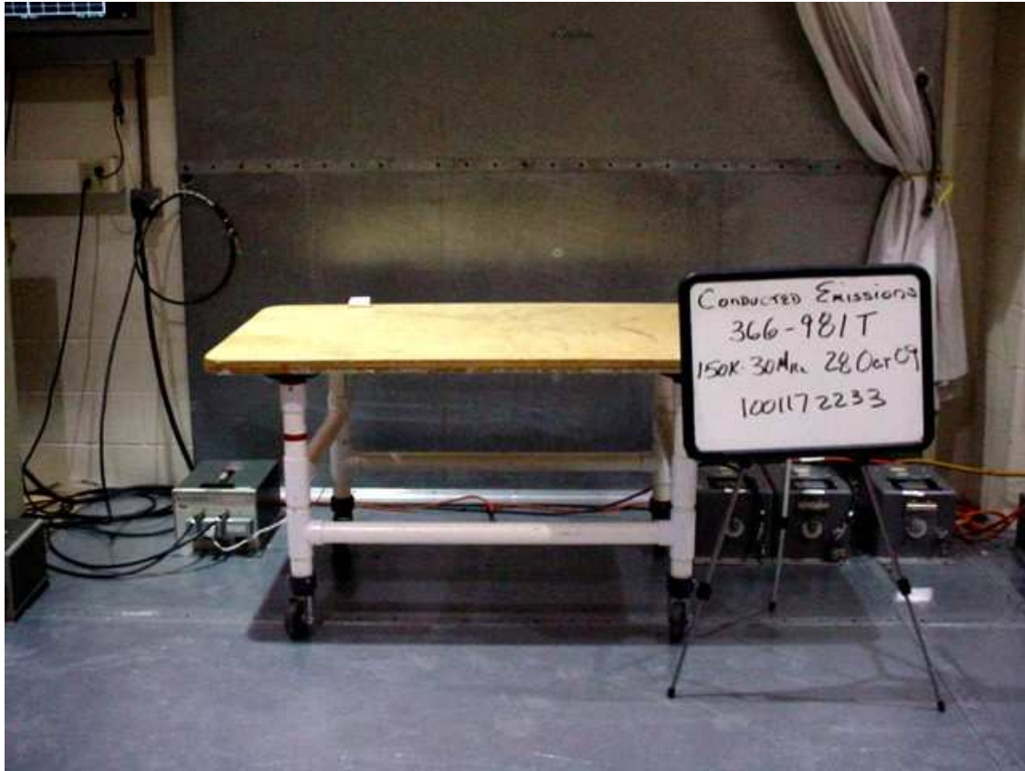
Figure 1 Test Setup for Conducted Emissions
