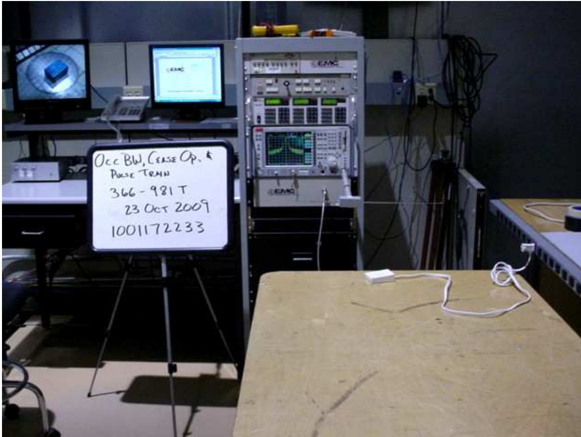
Figure 9 Test Setup for Cease Operation
