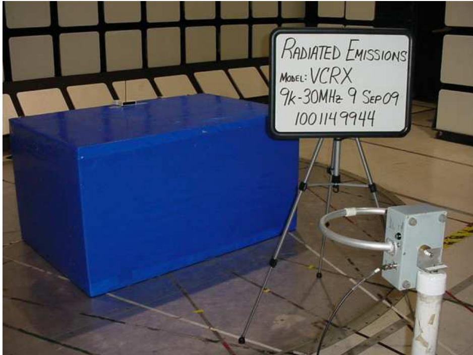
Figure 11 Test setup for Radiated Emissions
