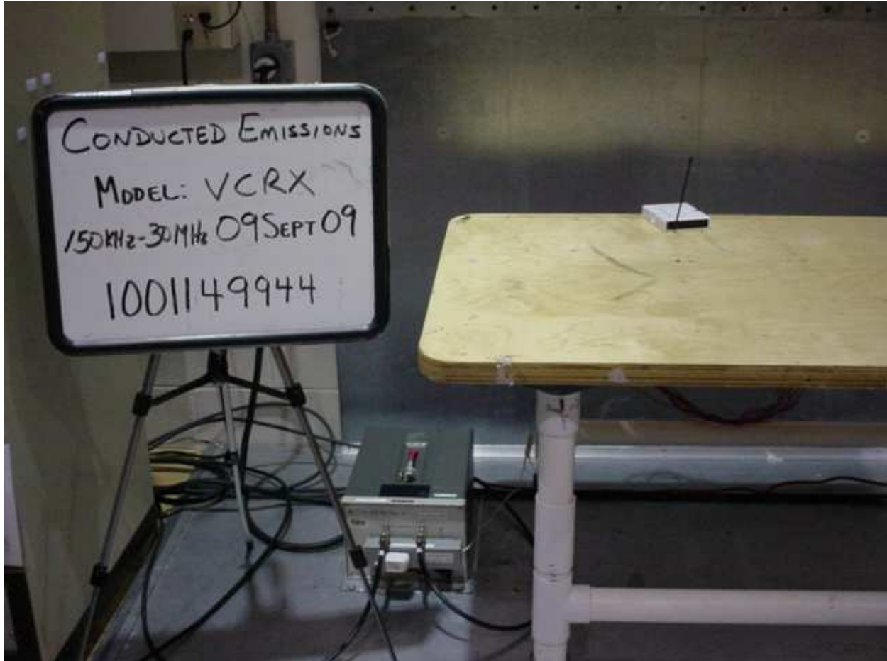
Figure 1 Test Setup for Conducted Emissions
