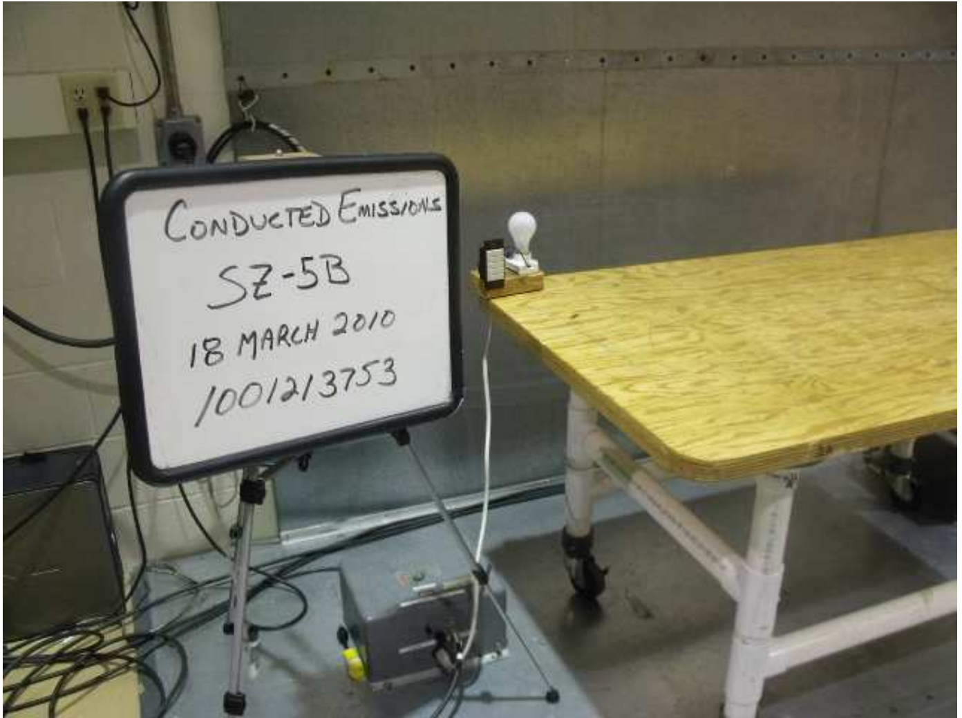
Figure 1 Test Setup for Conducted Emissions
