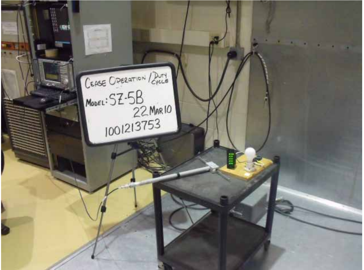
Figure 9 Test Setup for Cease Operation
