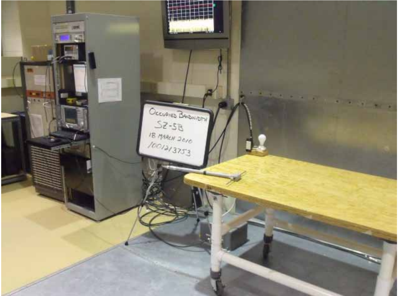
Figure 6 Test Setup for Occupied Bandwidth
