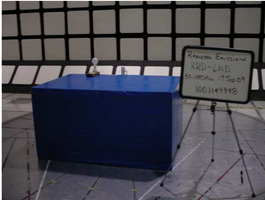
Figure 20 Test setup for Radiated Emissions
