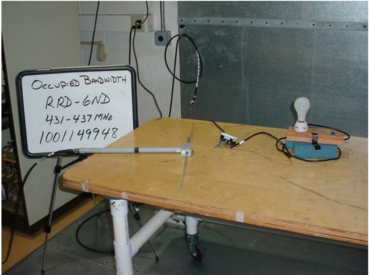
Figure 6 Test Setup for Occupied Bandwidth
