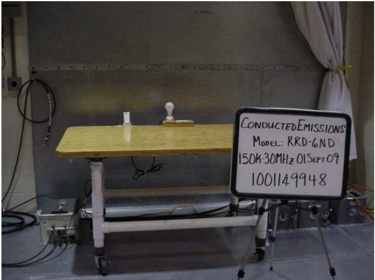
Figure 1 Test Setup for Conducted Emissions
