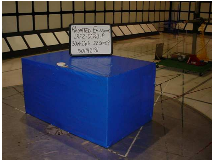
Figure 14 Test setup for Radiated Emissions
