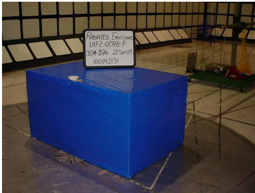
Figure 14 Test setup for Radiated Emissions
