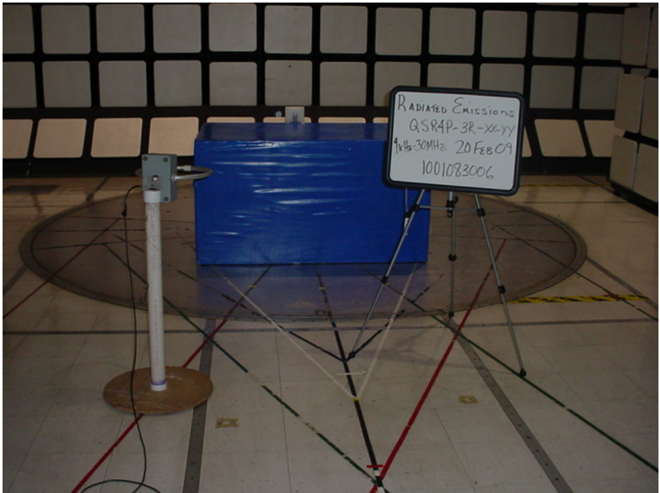
Figure 9 Test setup for Radiated Emissions
