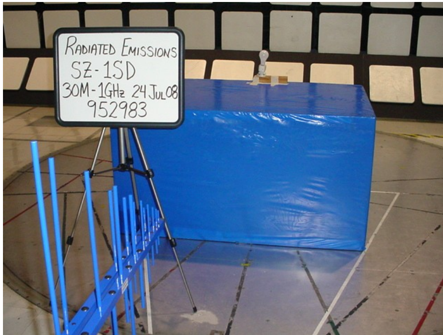
Figure 20 Test setup for Radiated Emissions (30-1000MHz Transmit Mode)
