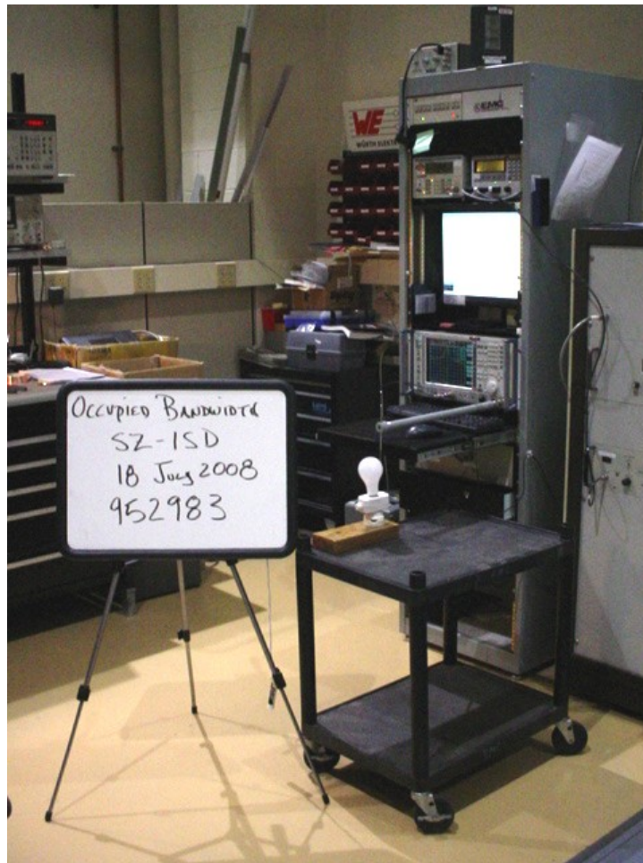
Figure 6 Test Setup for Occupied Bandwidth
