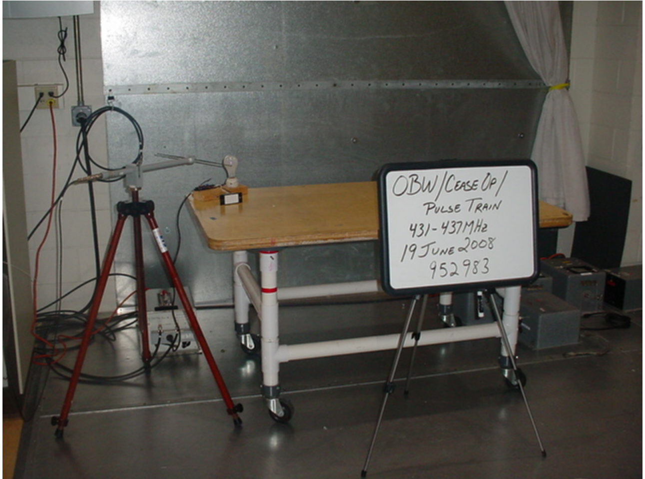
Figure 17 Test Setup for Cease Operation
