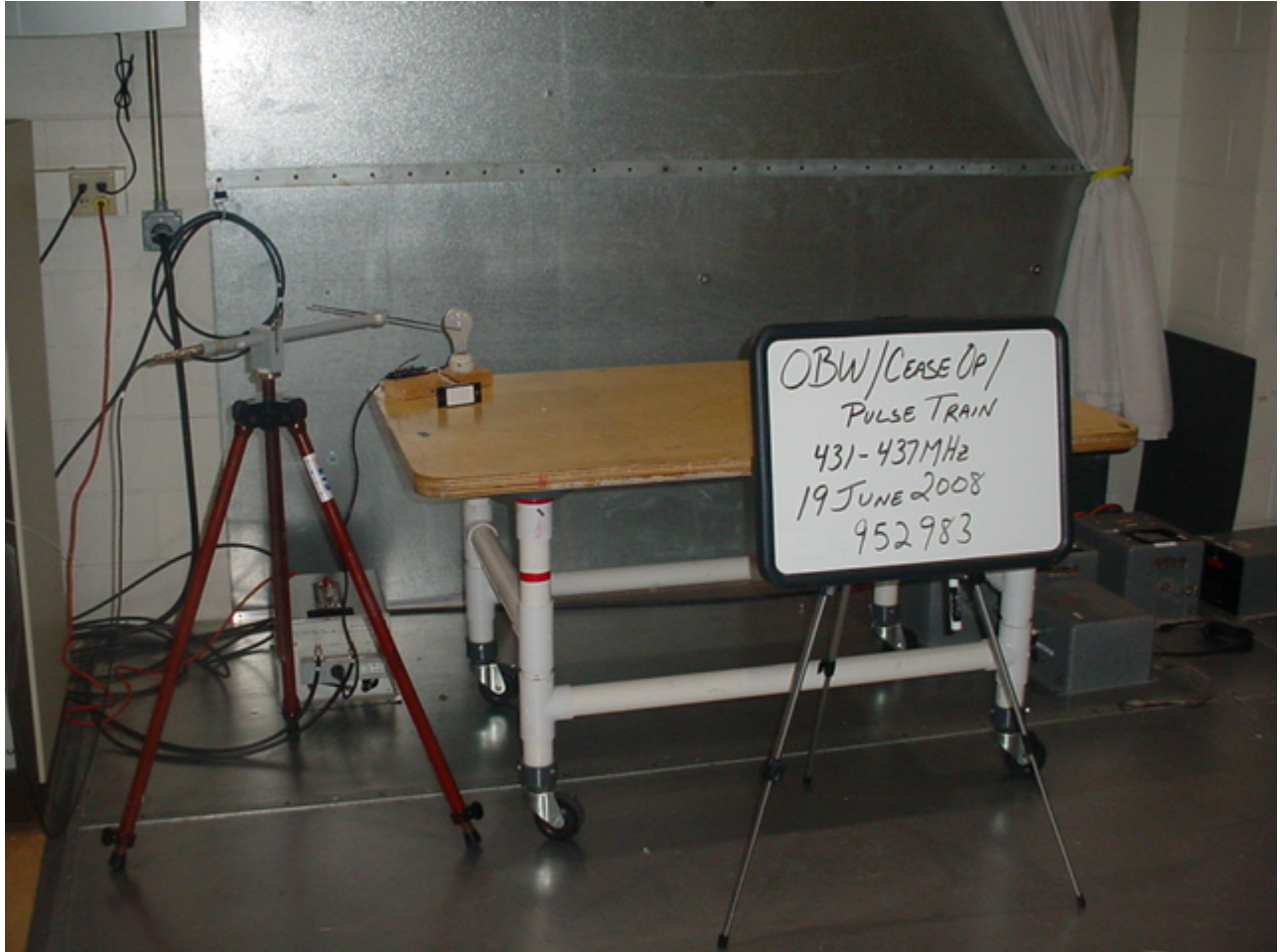
Figure 10 Test Setup for Occupied Bandwidth
