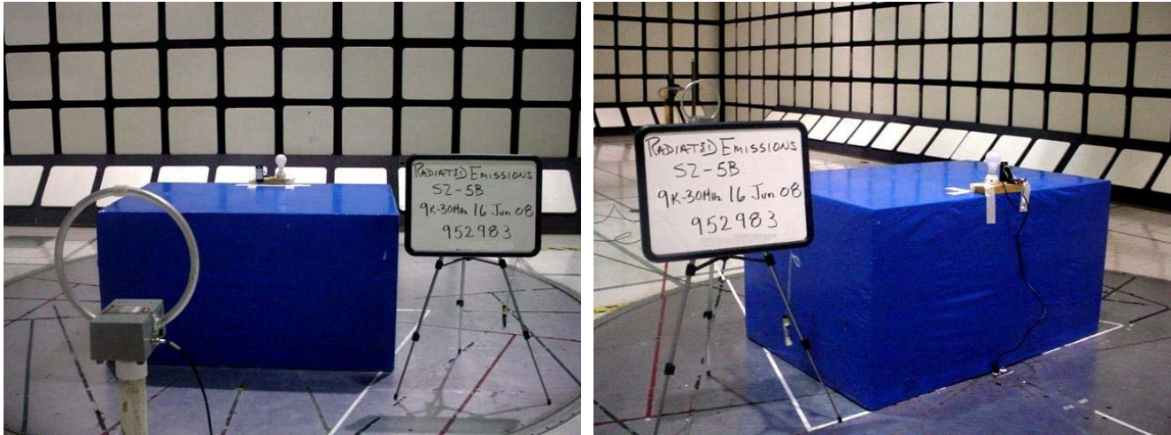
Figure 23 Test setup for Radiated Emissions 9kHz – 30MHz
