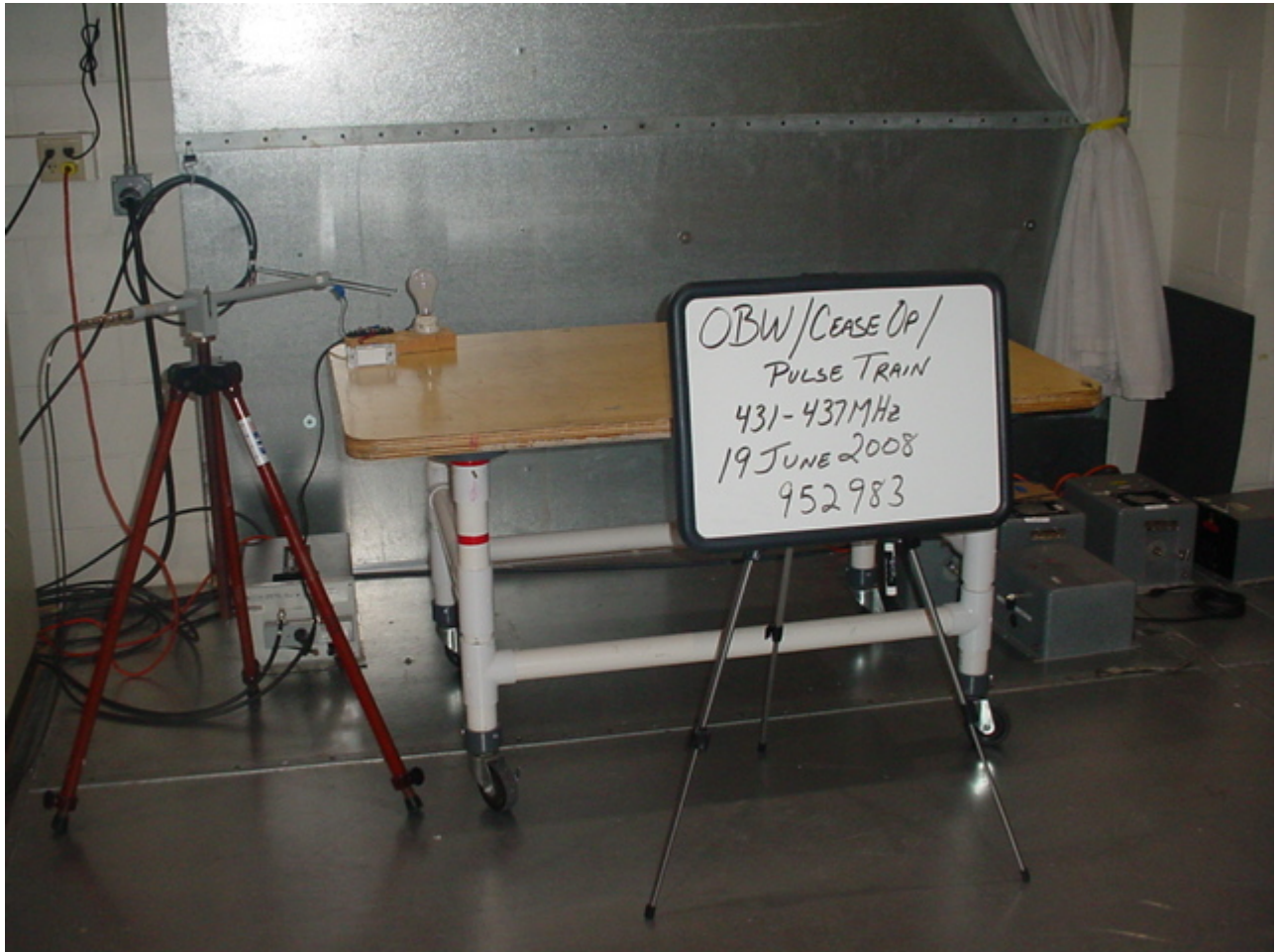
Figure 10 Test Setup for Occupied Bandwidth
