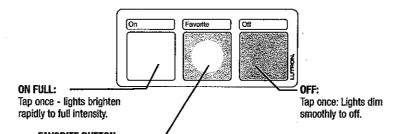
Tap once to recall your favorite light level. To store your favorite level, adjust rocker on dimmer, press and hold favorite button for about 8 seconds until the dimmer LED begins to cycle quickly. ("Off" is a valid preset level.)
