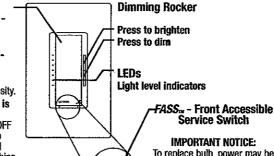
· Press and hold when unit is on - Each time dimmer is turned off delayed fade to OFF can be activated. As the tap button is held, the LEDs will begin to flash. The first flashing LED represents a 10 second fade to OFF. Each additional flashing LED represents an additional 10 seconds of delay before lights fade to OFF (up to 60 seconds of delay).
