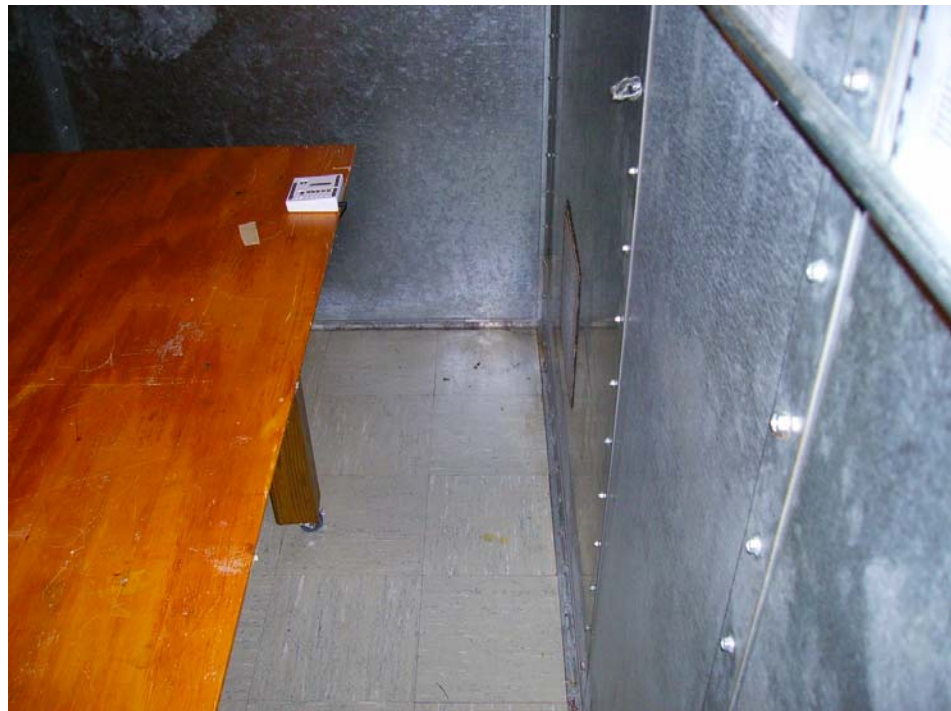
EUT 40cm from vertical ground plane
