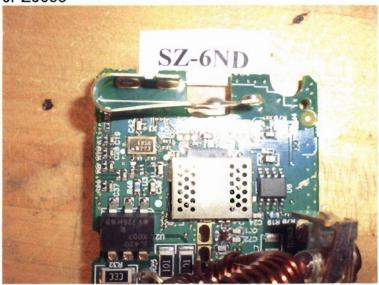
This model has the addition of an electronic lamp dimming circuit. The RF transceiver is relaid out to accommodate the dimming circuitry and a shield added to protect the transceiver from the dimming circuitry. The antenna is changed from a dipole to a loop antenna.
