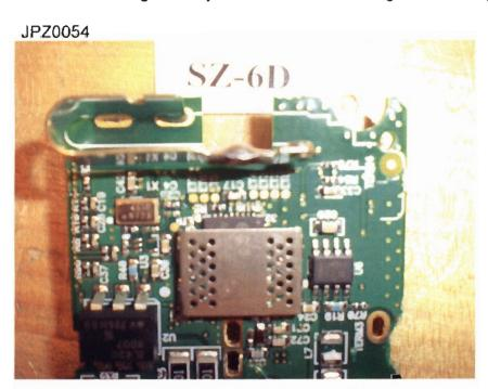
This model is the same JPZ0053 except the power supply is in series with the load.
