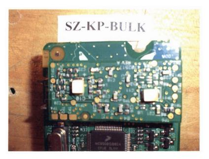
This model has the addition of push-button controls and the antenna is changed to a loop antenna.
