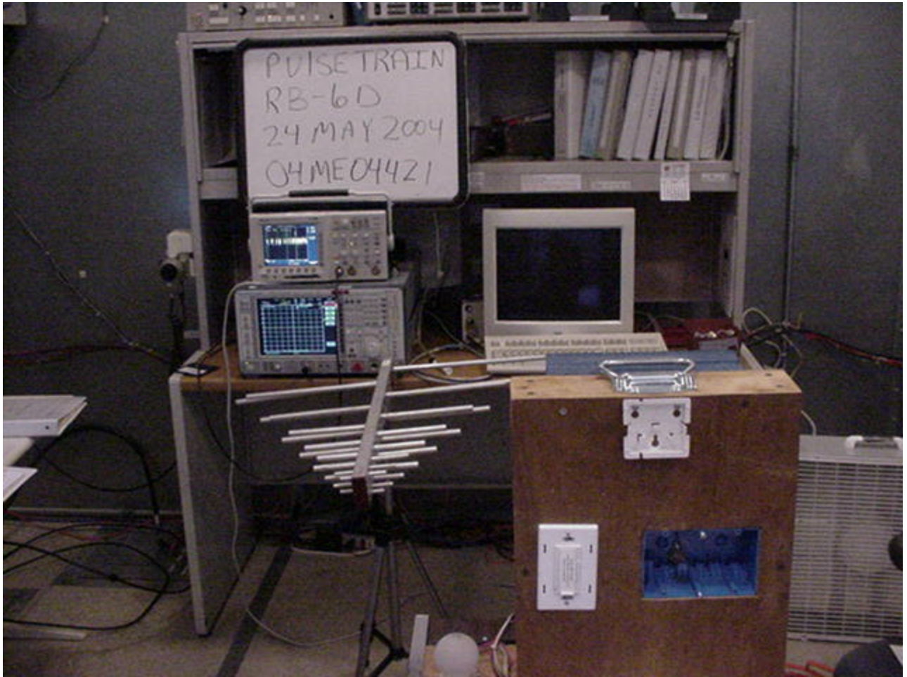
Pulse Train Test Set-Up
