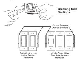
When removing side sections for multigang installations, reduction of the dimmer's load capacity is required. See table below.
