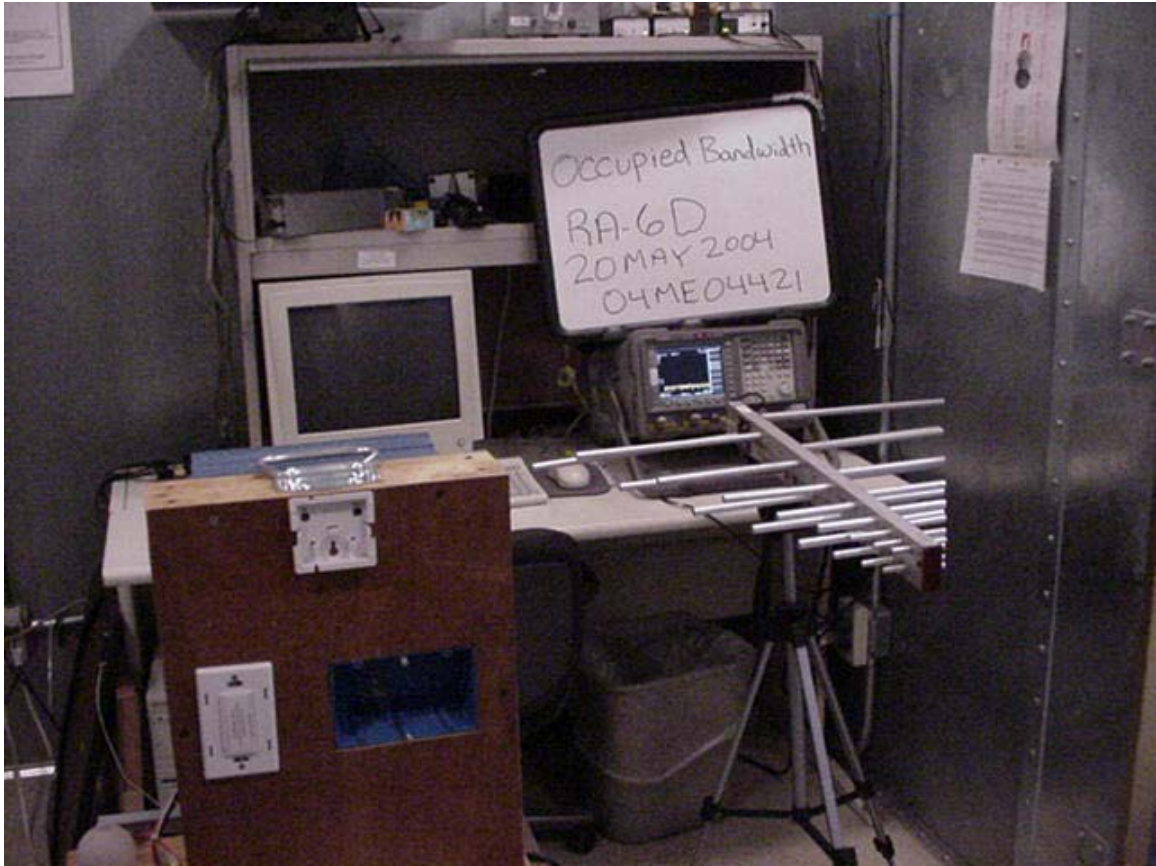
Occupied Bandwidth Test Set-Up
