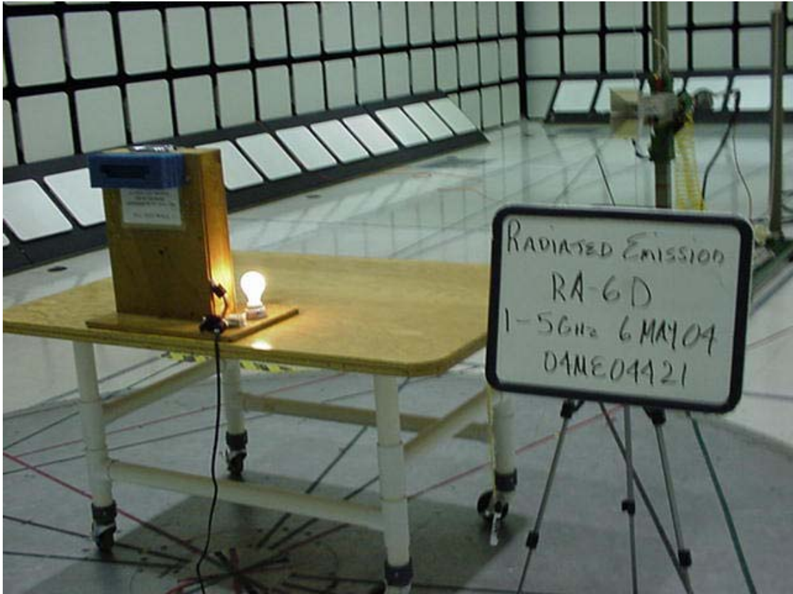
Radiated Emission Test Set-up Rear View 1 -5GHz
