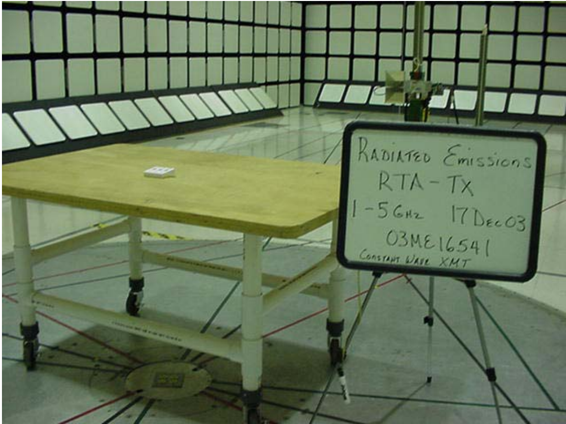
Radiated Emission Test Setup 1GHz to 5GHz Rear View
