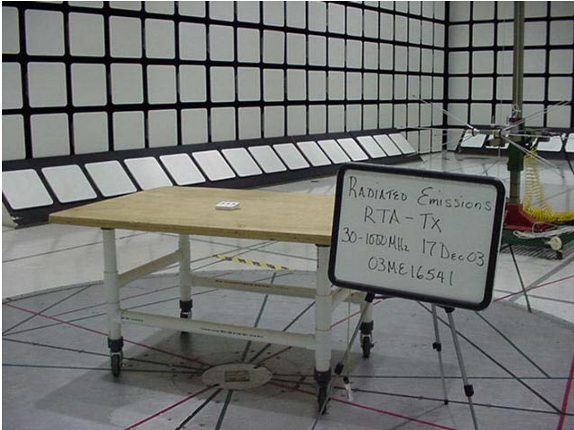
Radiated Emission Test Setup 30MHz to 1000MHz Rear View
