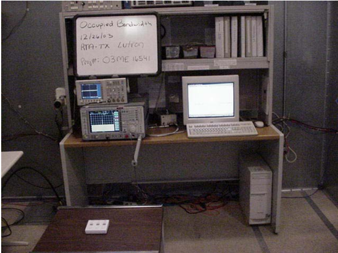
Occupied Bandwidth Test Set-Up
