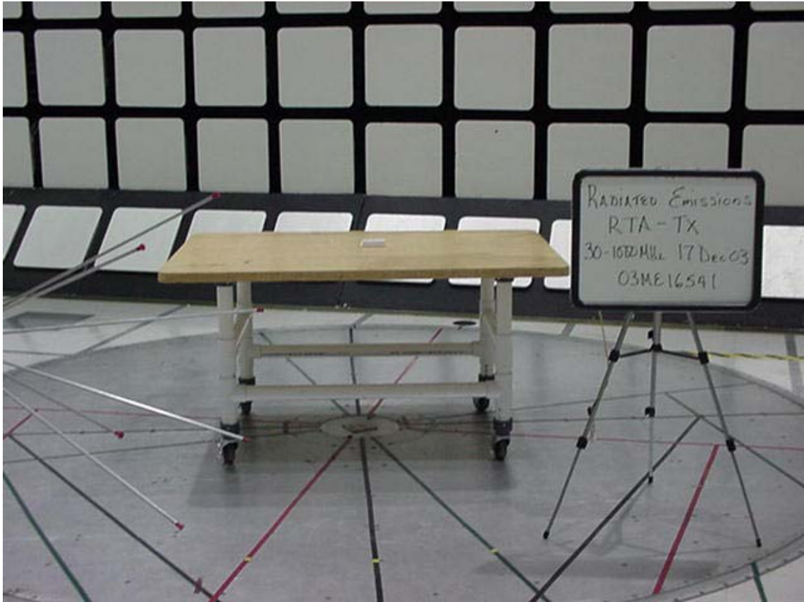
Radiated Emission Test Setup 30MHz to 1000MHz Front View
