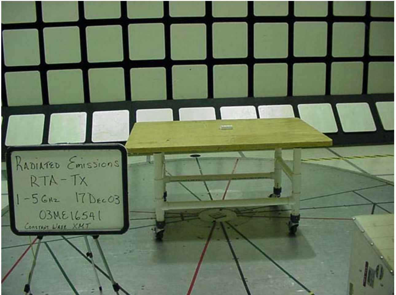
Radiated Emission Test Setup 1GHz to 5GHz Front View
