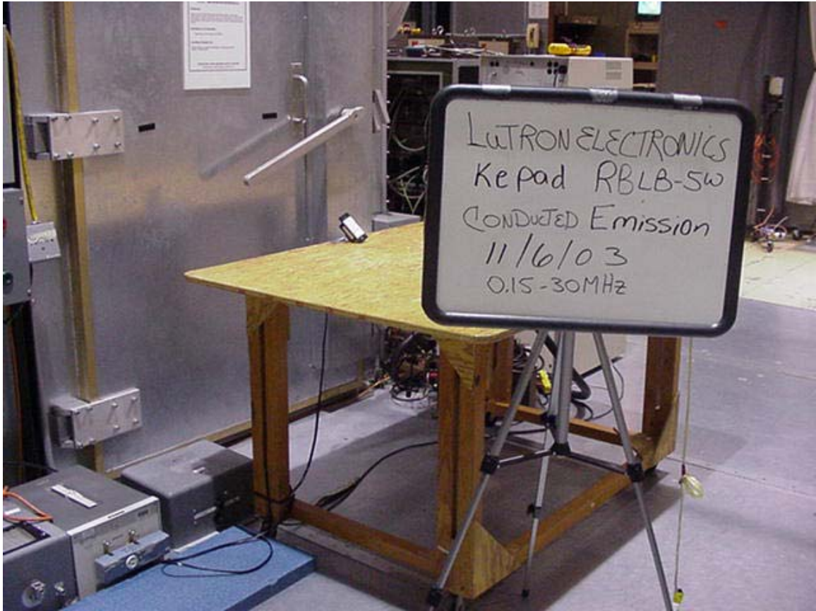
Conducted Emission Test Set-Up
