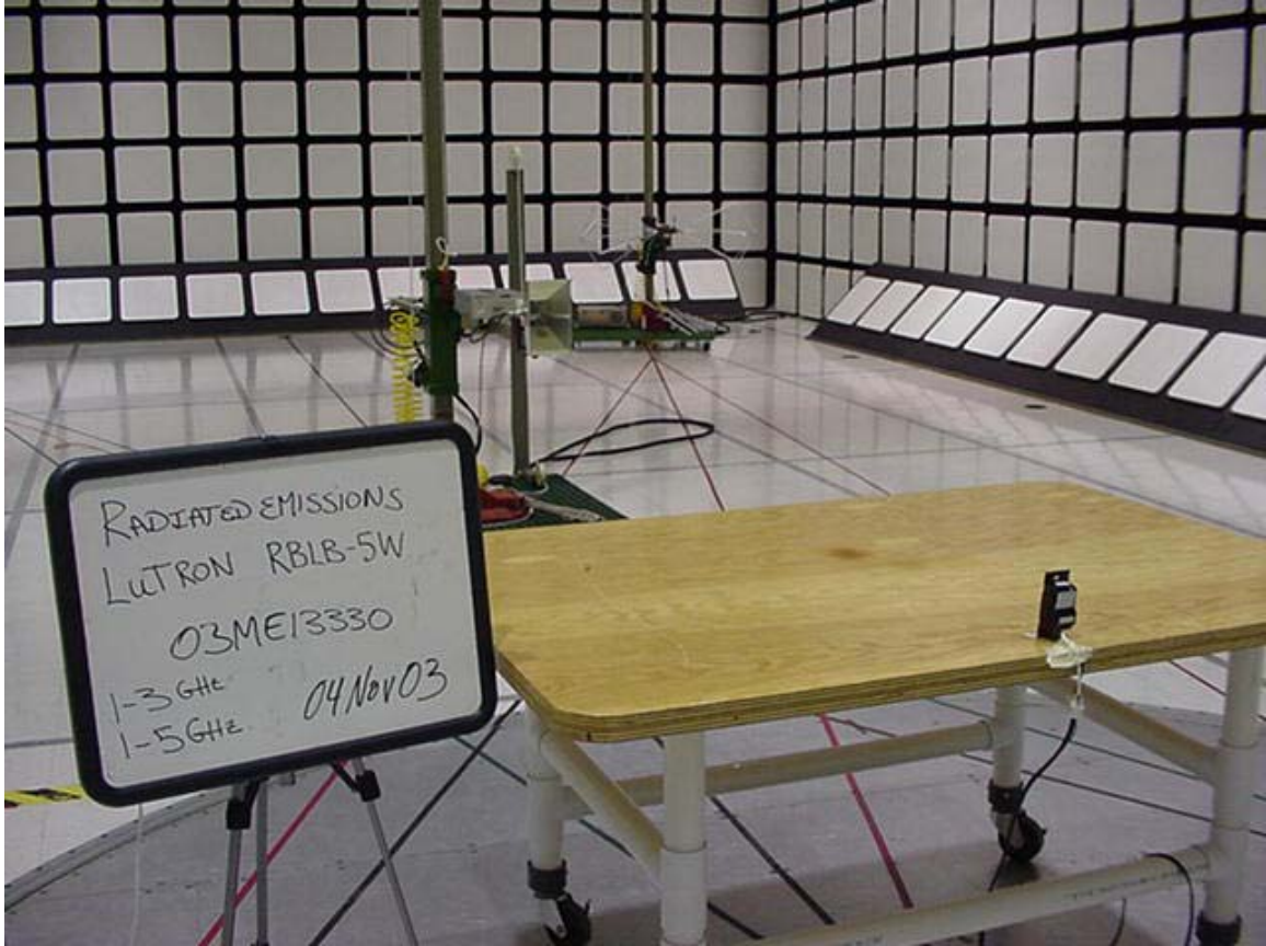
Radiated Emission Test Set-Up 1-5GHz Rear View
