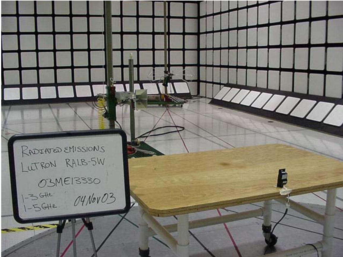
Radiated Emission Test Set-Up 1-5GHz Rear View
