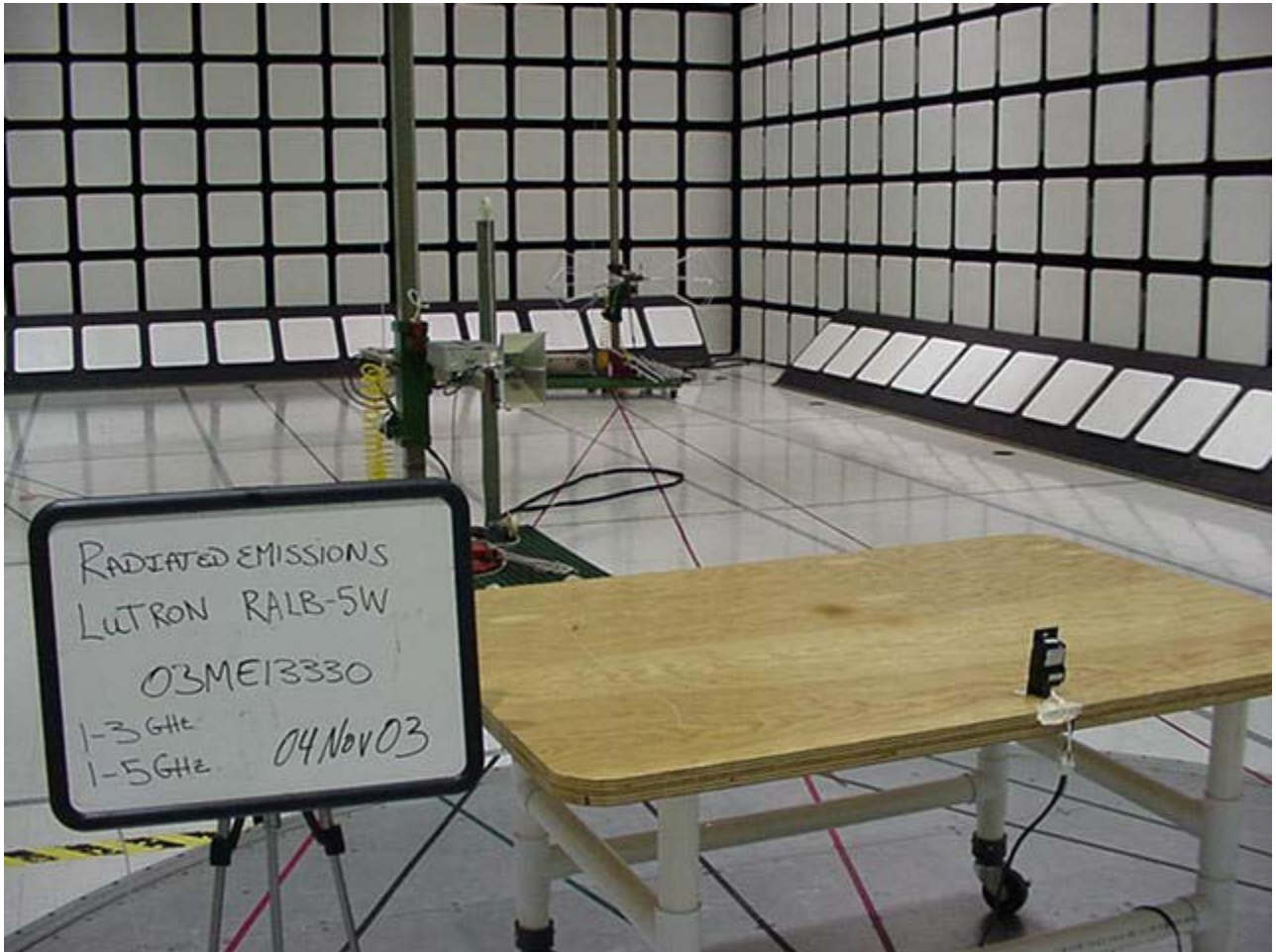
Radiated Emission Test Set-Up 1-5GHz Rear View
