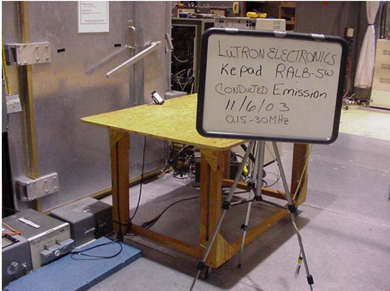
Conducted Emission Test Set-Up
