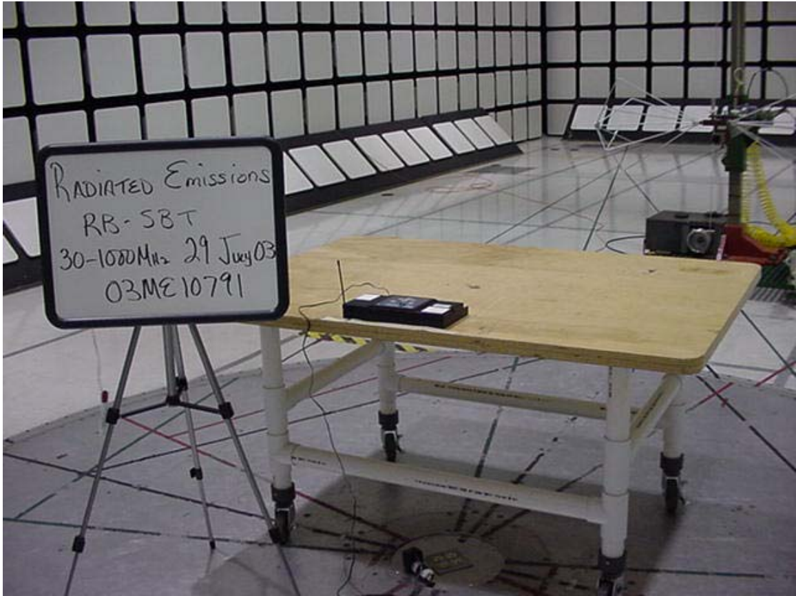
Radiated Emissions Test Set-Up 30-1000MHz Rear View
