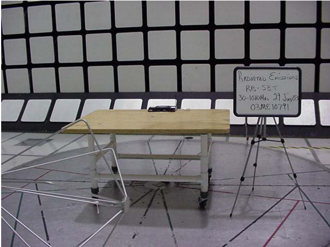
Radiated Emissions Test Set-Up 30-1000MHz Front View
