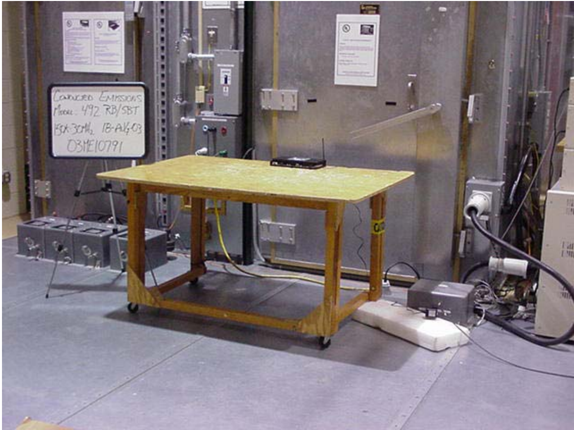
Conducted Emission Test Set-Up 150KHz to 30 MHz
