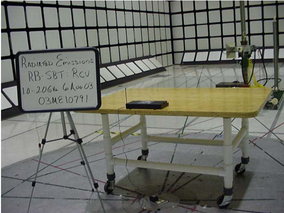
Radiated Emissions Test Set-Up above 1GHz Rear View
