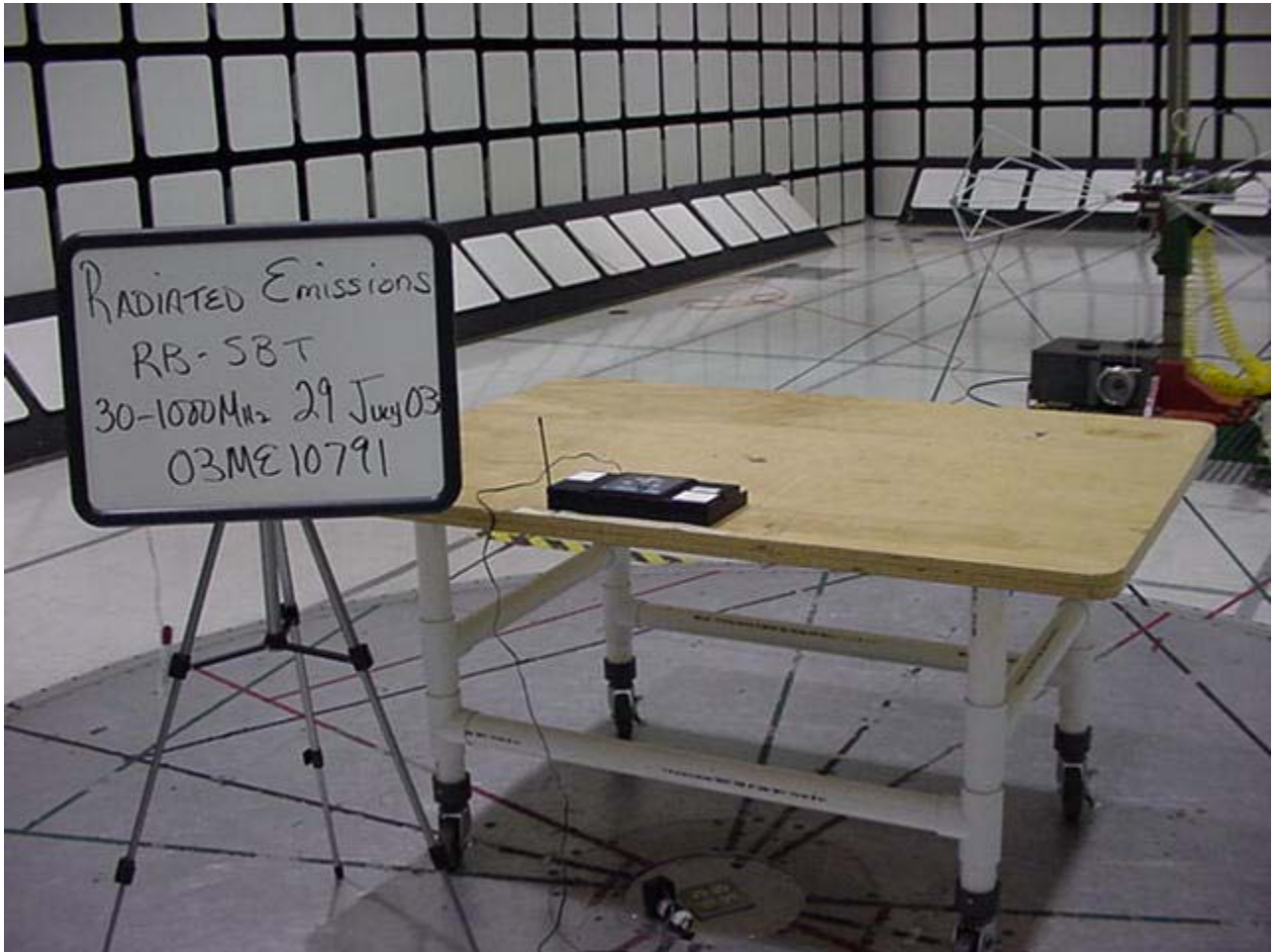
Radiated Emissions Test Set-Up 30-1000MHz Rear View
