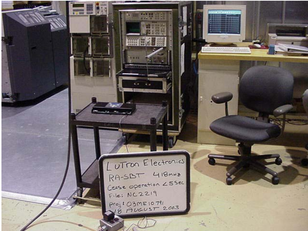
Cease Operation in Less Than 5 seconds Test Set-Up Note: The test photo depicted states RA-SBT 418 MHz. This is actually the RB-SBT, which operates at 433.9 MHz
