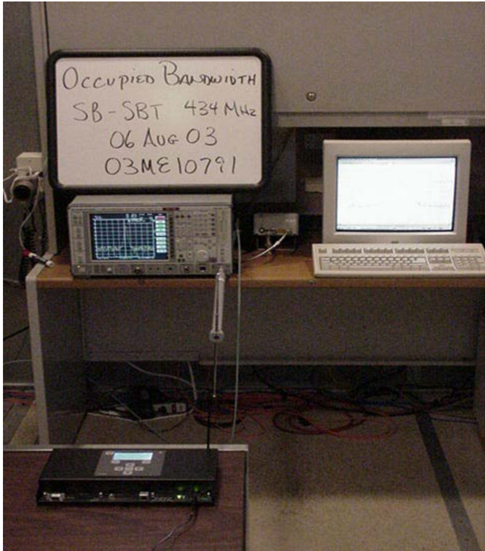
Occupied Bandwidth Test Set-up
