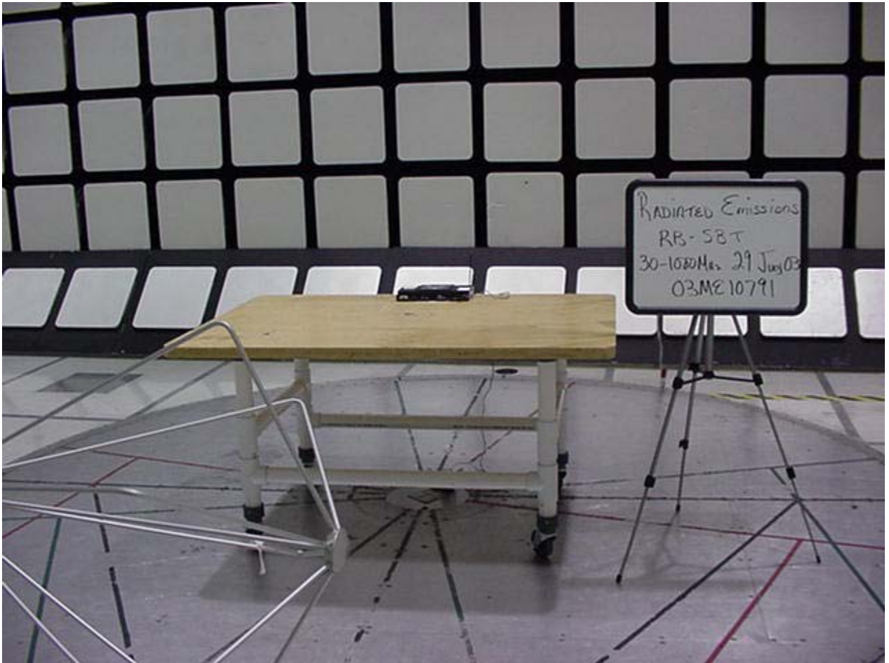
Radiated Emissions Test Set-Up 30-1000MHz Front View
