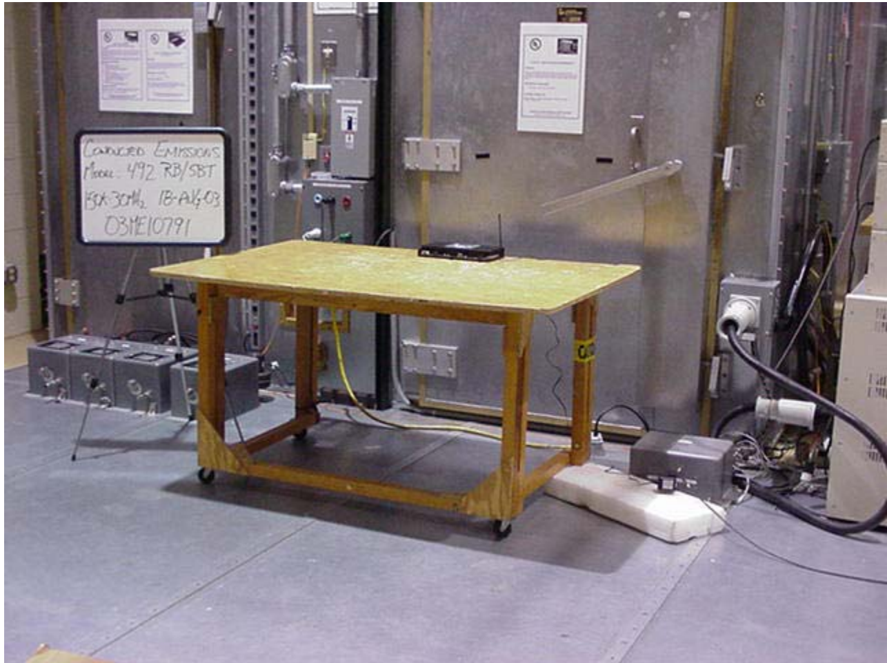
Conducted Emission Test Set-up 150KHz to 30MHz
