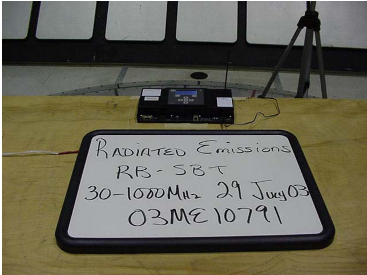
Radiated Emissions Test Set-Up
