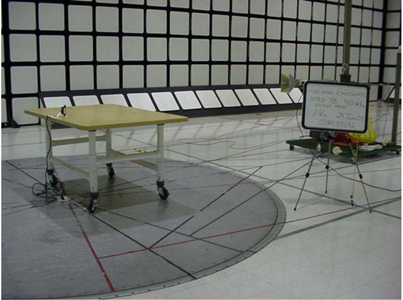
Radiated Emission Test Set-Up 1-2GHz Rear View
