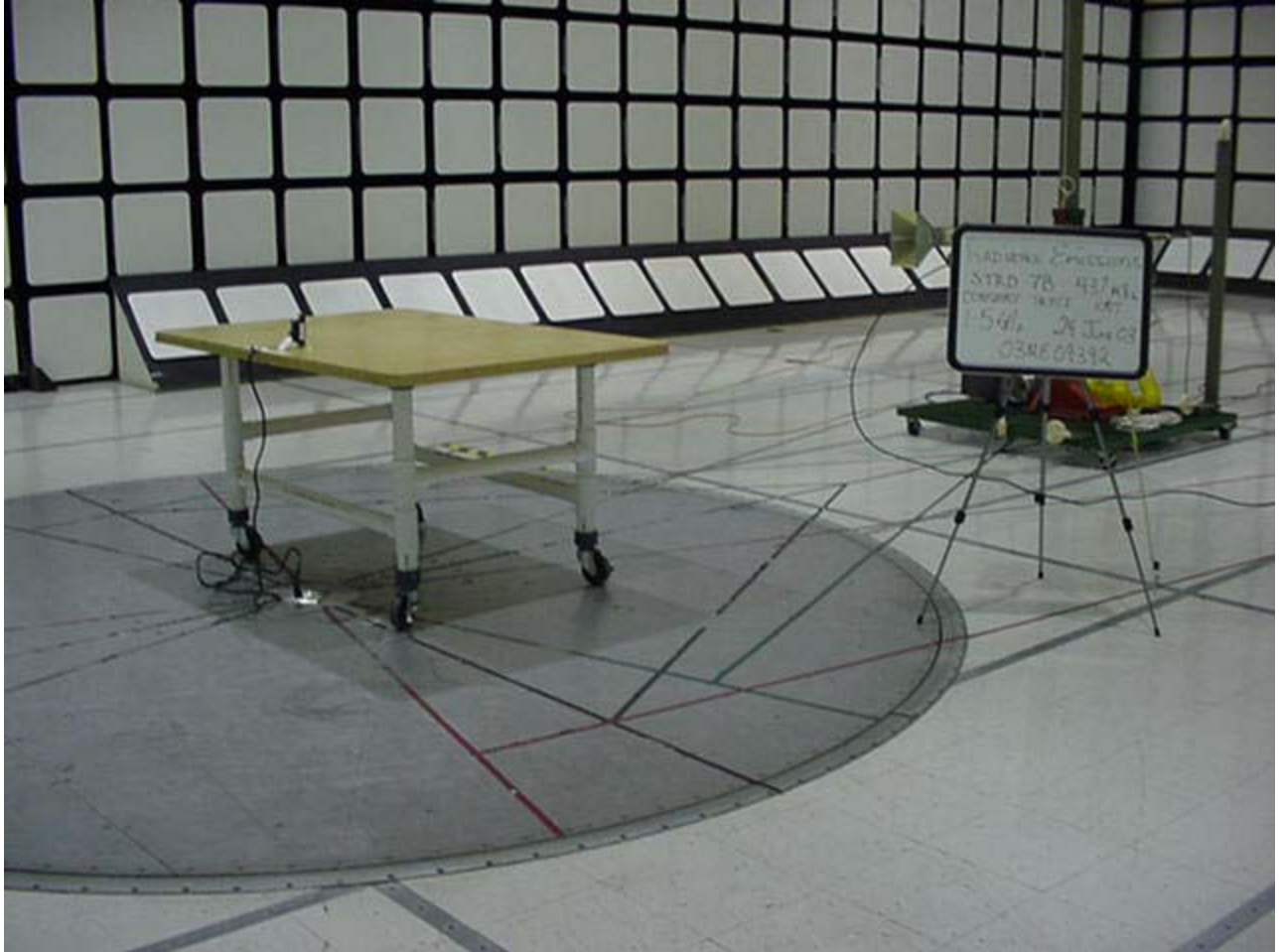
Radiated Emission Test Set-Up 1-5GHz Rear View
