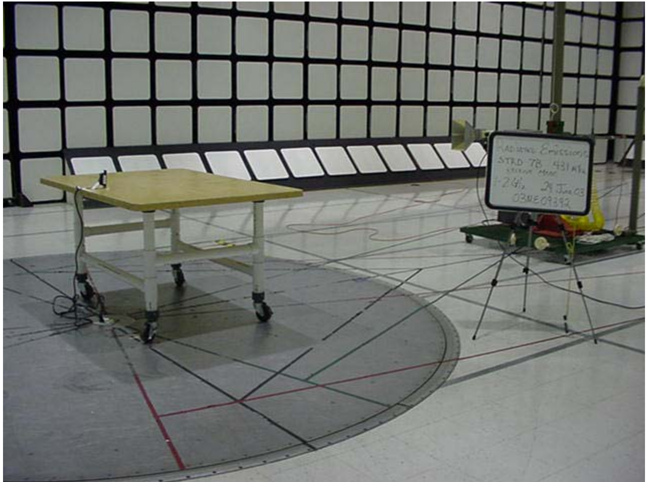
Radiated Emission Test Set-Up 1-2GHz Rear View
