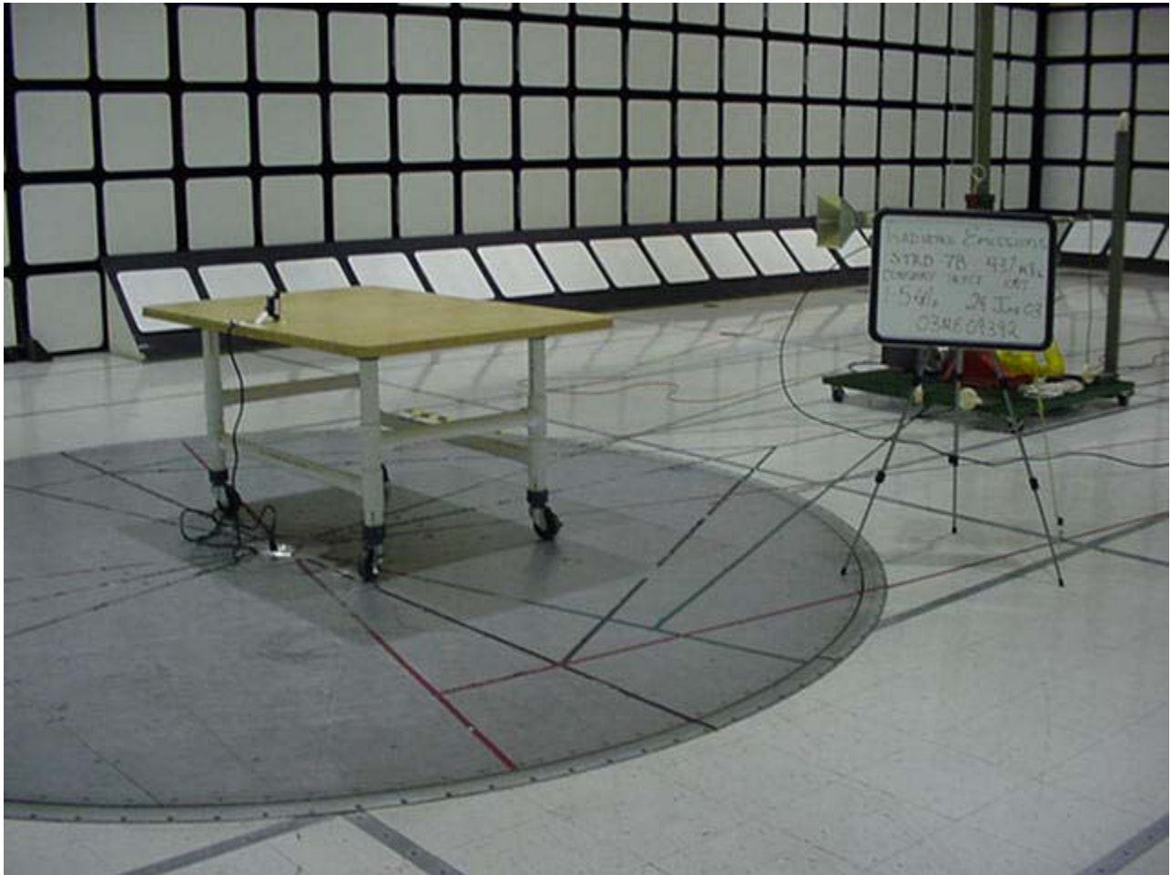
Radiated Emission Test Set-Up 1-5GHz Rear View
